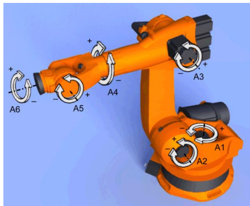
Figure 2: The scheme of rotation around the individual axes.
